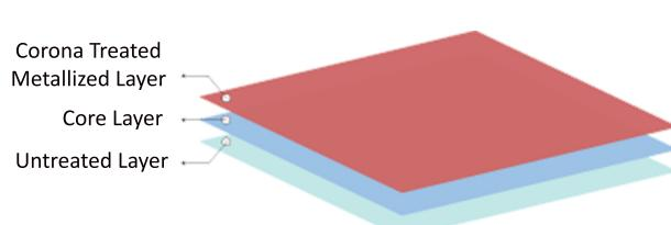
Is a metallized co-extruded BOPET film, with one side corona treated and other side untreated
